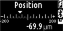
Figure 12. pickup tip position display screen.
