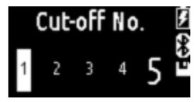
Figure 8. cut-off length setting screen.
