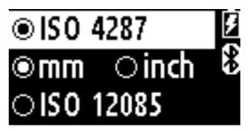
Figure 6. measurement standard setting screen.
